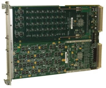
Figure 3 - Talon Instruments T940 50 MHz Digital Instrument from EADS North America Test and Services
